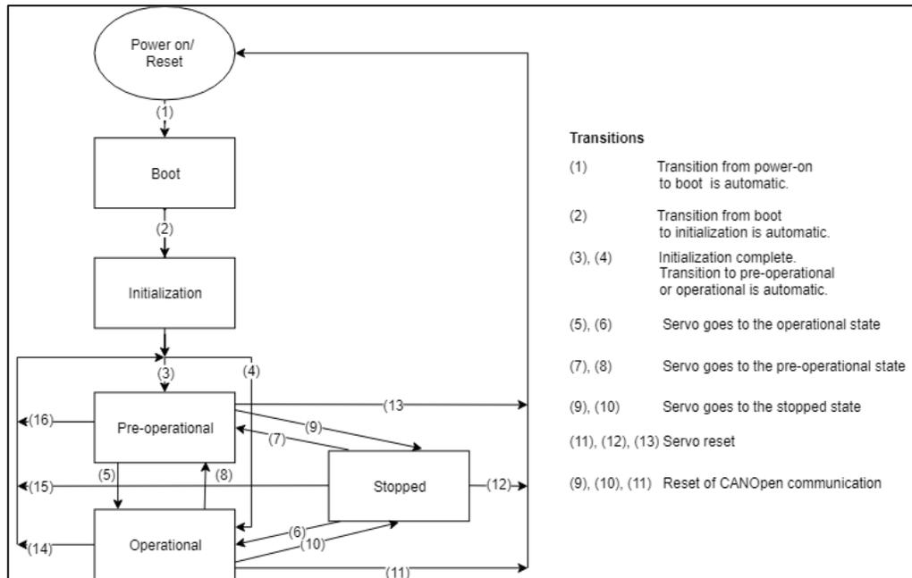
**Figure 1-5: State transition diagram for RDrive servos**
