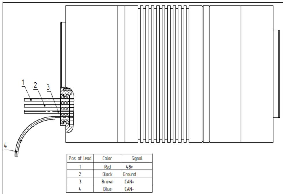
**Figure 1-1: Cable gland with CAN wires on the rear mounting flange**
