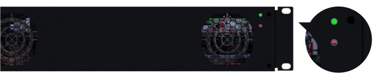
When the red LED on the control box lights up, this indicates an error. Flip the power switch on the control box into the "OFF(0)" position and wait for the indicators on the front panel to go off completely. Then, make sure the emergency shutdown button is unpressed and the Step 2 connections are correct and secure, switch the arm back on.
