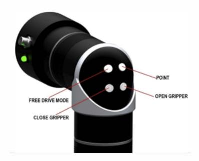
In the Free Drive mode, the arm cannot retain its position stably. Therefore, when you work with the arm in the mode, make sure to support it with your hands.
