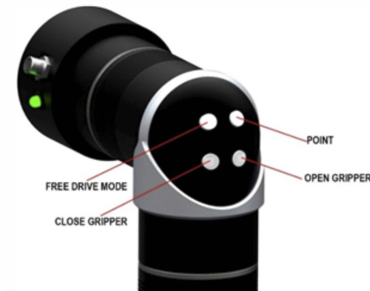
In the Free Drive mode, the arm cannot retain its position stably. Therefore, when you work with the arm in the mode, make sure to support it with your hands.
