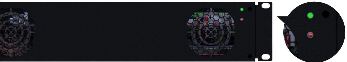
When the red LED on the control box lights up, this indicates an error. Flip the power switch on the control box into the “OFF(0)” position and wait for the indicators on the front panel to go off completely. Then, make sure the emergency shutdown button is unpressed and the Step 2 connections are correct and secure, switch the arm back on.
