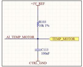
Figure 1-2: NTC thermistor interface in FMI motors
