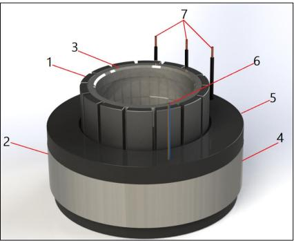
Figure 1-1: Rotor and stator assemblies with cable outputs
