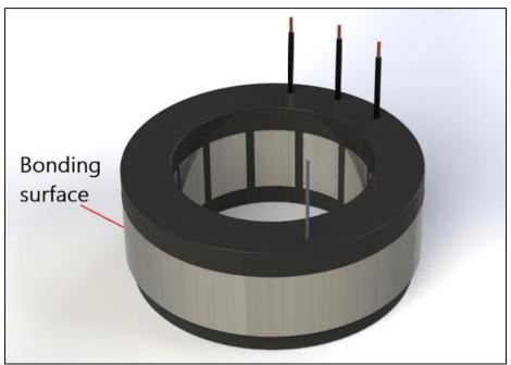
Figure 3-1: The bonding surface of a stator
